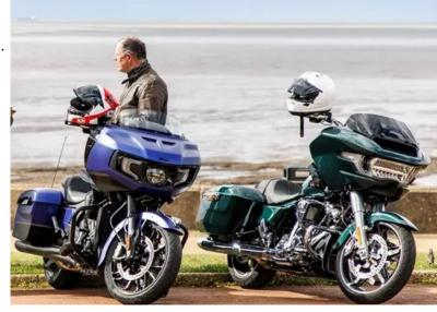
Suspension F:43mm inverted forks, non-adjustable. R: Monoshock, adjustable (optional electronically) Front brake 2 x 320mm discs with four-piston Brembo radial calipers. Cornering ABS Rear Brake 1x298mm disc with two-piston caliper. Cornering ABS Seat Height 26.5", Curb Weight 840 Lbs.
